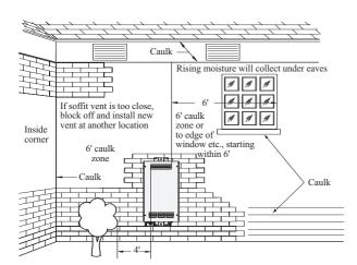
AWARNING: Moisture in the flue gas will condense as it leaves the vent terminal. In cold weather this condensate can freeze on the exterior wall, under the eaves and on surrounding objects. Some discoloration to the exterior of the building is to be expected. However, improper location or installation can result in severe damage to the structure or exterior finish of the building
